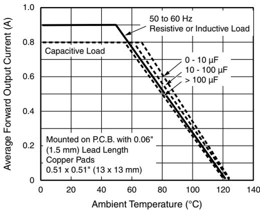
Fig. 2 - Derating Curves Output Rectified Current for B250C800D...B360C800DM
