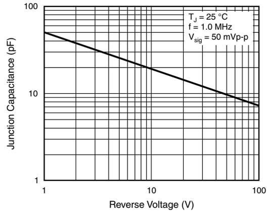
Fig. 6 - Typical Junction Capacitance Per Diode
