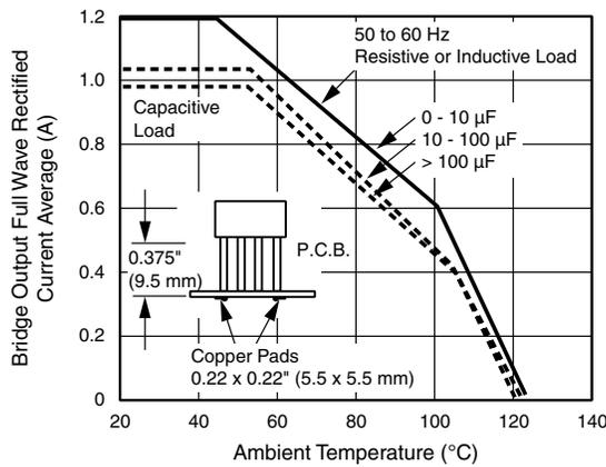
Fig. 1 - Derating Curves Output Rectified Current for B40C1000G...B125C1000G
