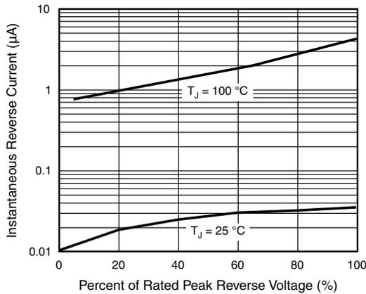
Fig. 5 - Typical Reverse Characteristics Per Diode
