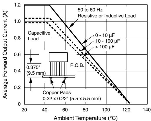
Fig. 2 - Derating Curves Output Rectified Current for B250C1000G...B380C1000G
